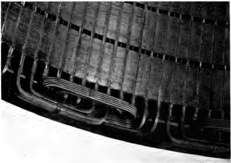
FIG. 253. —Three-phase, Half-coiled, Double-coil, Two-slot Spiral Winding in three ranges (six-phase grouping).
